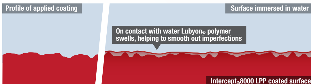
Coating swelling on immersion
